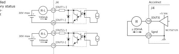
When configured as a Custom function, the output will go active when any of the events becomes true. When active, the output can be configured as on or off. The output can also be set to latching, or non-latching.
